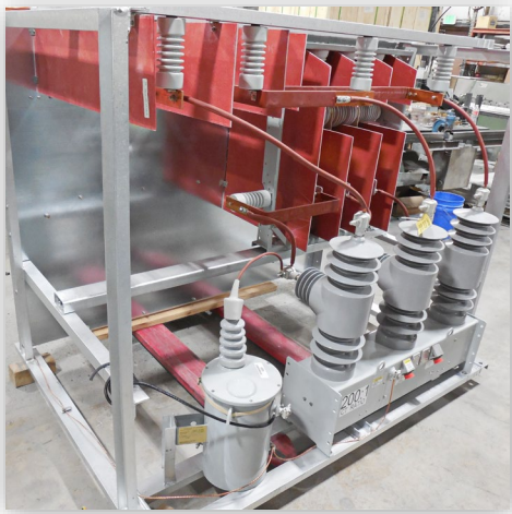
Three-phase, electronically controlled, vacuum-interrupting automatic circuit recloser and 1 KVA control power transformer
