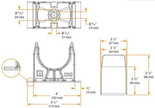
Tabs on both sides control spacing between saddled components. Designed to break easily at the "V" notch on both ends if necessary.
